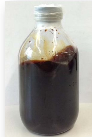
oxyalkylated liquefied lignin = modified
