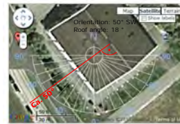
Fig. 2 Roof characteristics of building on which PV modules are installed
