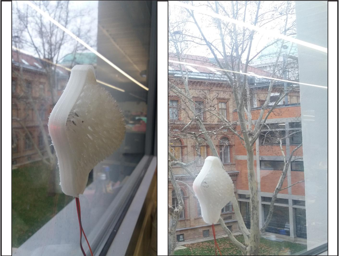
The idea is to make sure the air ventilates properly and no one can touch it as the sensors get quite hot. The outdoor sensor is to be protected by the rain while still guaranteeing a good ventilation
