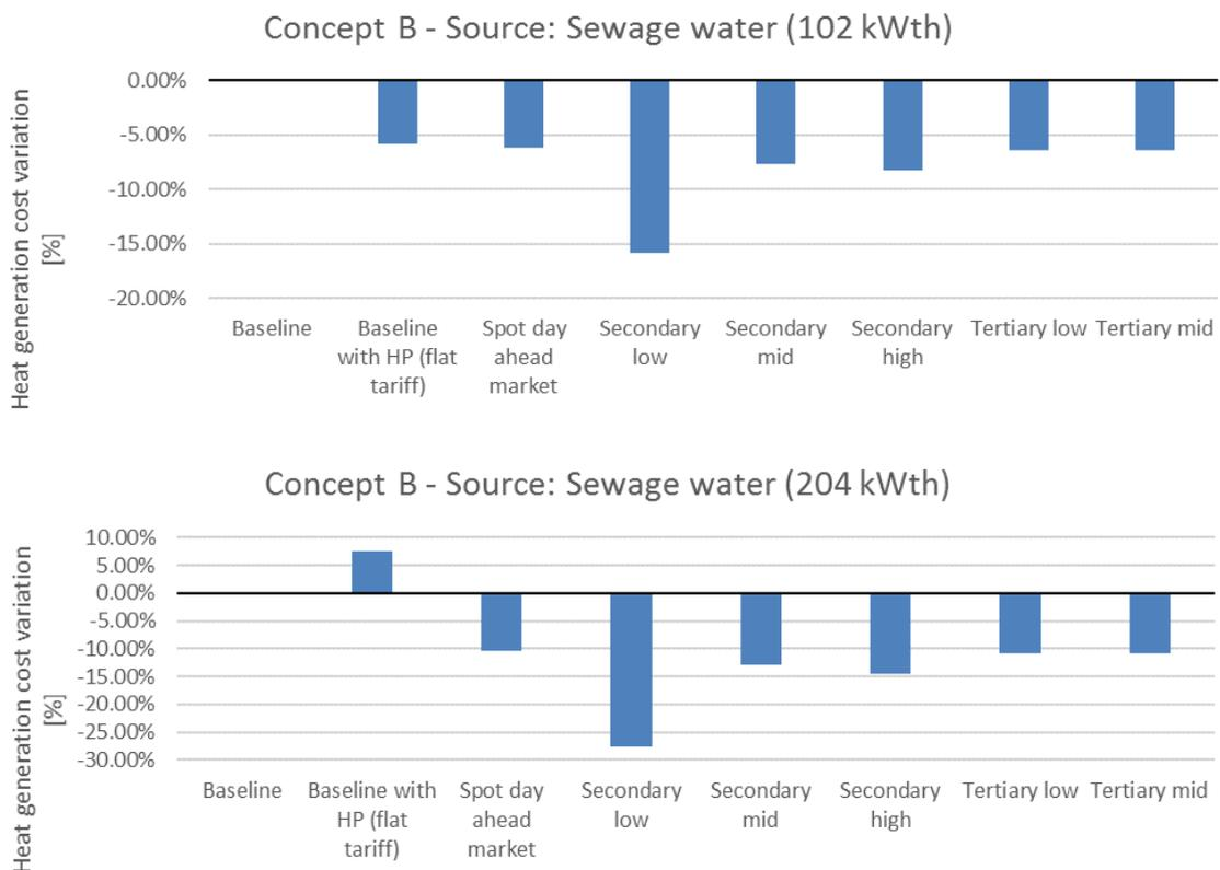
Figure 12: variation in the annual heat generation costs for the use cases with sewage water as a source for the heat pump
