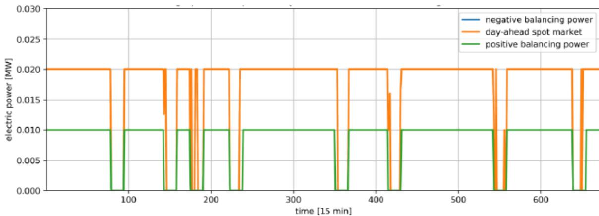
Figure 4: “high” bidding strategy for the heat pump (1 week). Use case: B3.1-SW.
