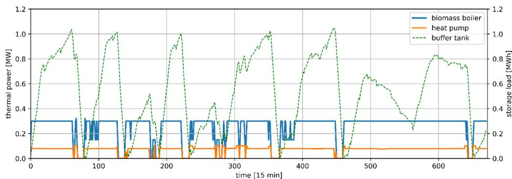
Figure 1: optimal operation of the biomass boiler, heat plant and storage for 1 week (15-minutes basis time step). Use case: B3-FG.
