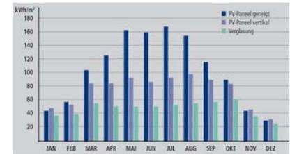
The folded façade allows efficient shading, optimized daylighting, +30% more Solar PV-Electricity Generation
