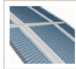
Micro sunshading louvers are highly specular systems that are installed in horizontal or slightly inclined glazings (glazed roofs or skylights). They are efficient sun shading solutions with SHGCs around 10-15% while providing daylighting from diffuse skylight and visual contact to the outside.
