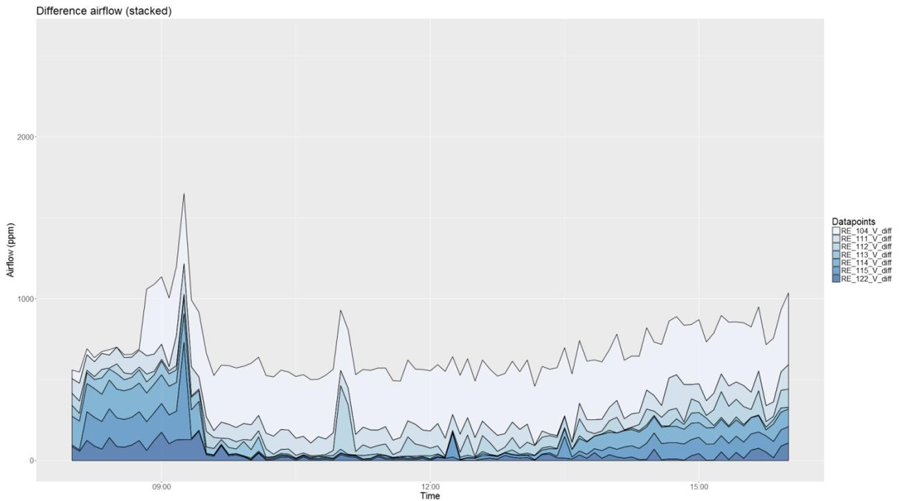
Figure 8 Cumulative difference between needed and provided airflows
