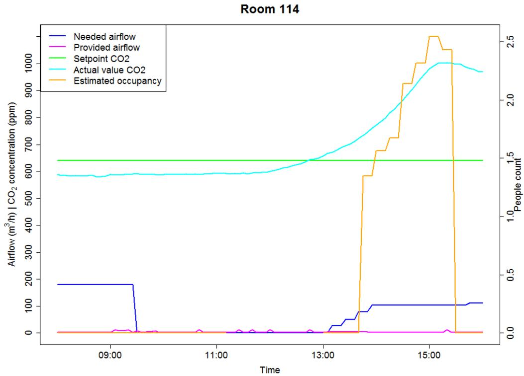
Figure 4 Airflow and CO<sub>2</sub> concentration (Room 114)
