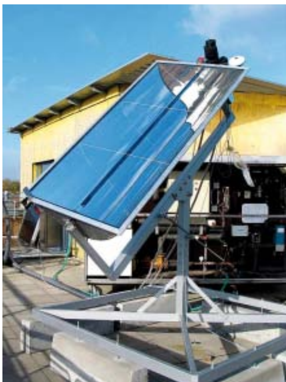
Testing of the PTC 1000 at the SIJ
