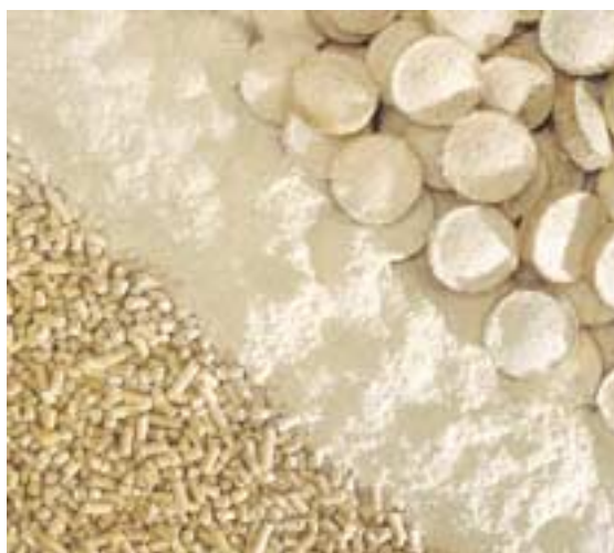
Pellets and briquettes made from sawdust are more suitable for transport than biomass raw materials which are often bulky and of low calorific value (Courtesy BrikettEnergi, Sweden)
