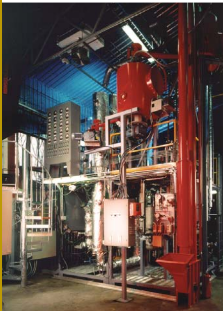
Figure 4: 20 kg/h fast pyrolysis process development unit at VTT
