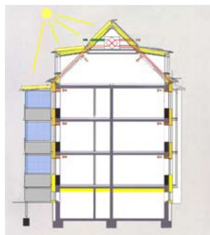
Prefabricated system renovation
