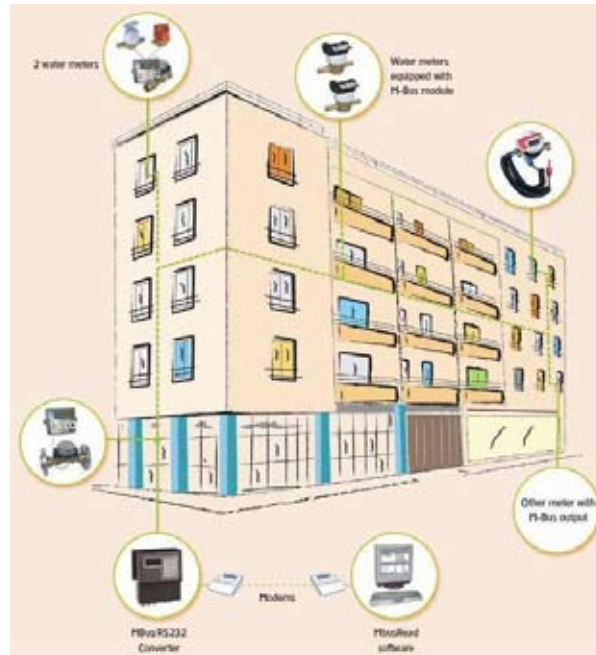
Deployment of energy metering in a commissioning project
