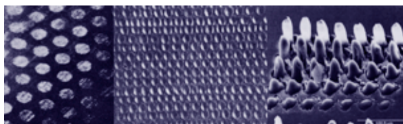
Examples of surface texture designs that reduce engine friction.
