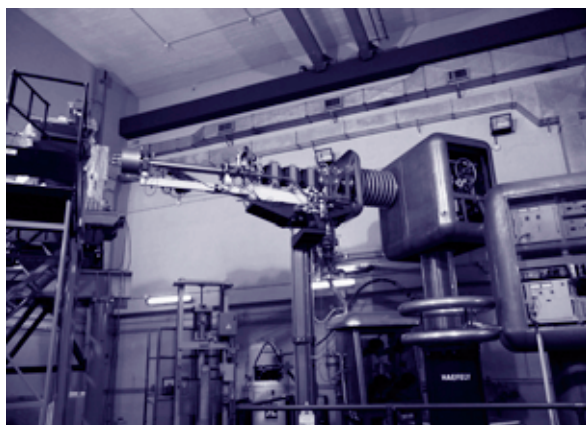
A 14-MeV fusion neutron irradiation facility, FNG (Frascati Neutron Generator), for the neutronics experiments of breeding blanket mock-ups.
