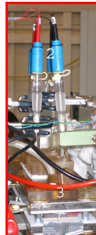
Single cell test apparatus fitted with four reference electrodes
