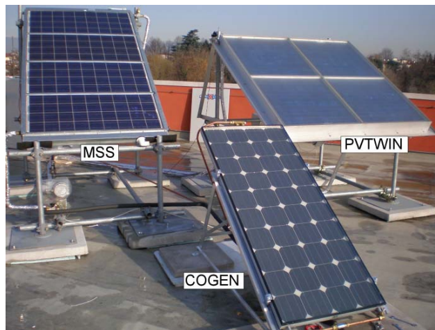
Figure 1. PV/T test stand at the University of Padova in Italy.
