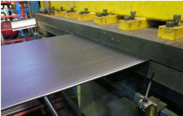
Extrusion of the Twin-wall sheet for the Aventa absorber.
