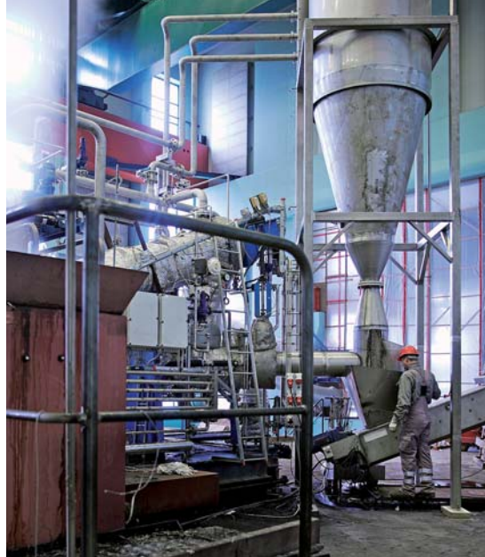
C5/C6 sugar and lignin platform biorefinery for ethanol, animal feed, power and heat from lignocellulosic residues. Courtesy Inbicon IBUS, Denmark; and Task 42.
