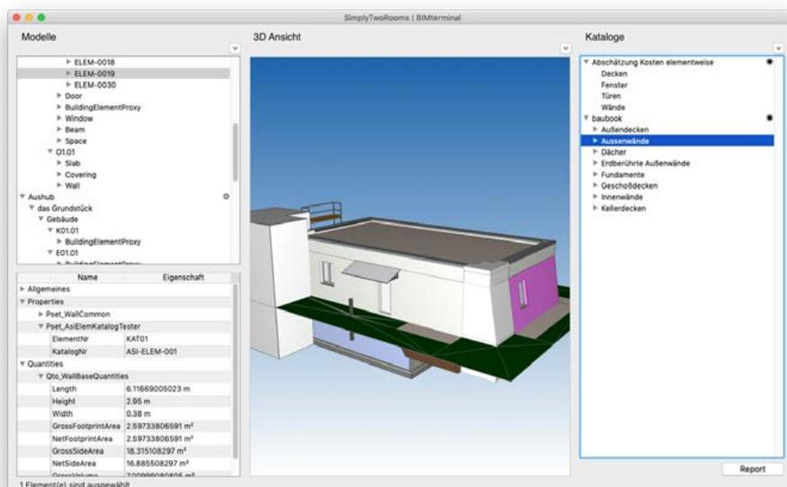
*The user interface is divided into three sections (left to right): Data browser with various different data views for the contents of the model / 3D geometrical images based on the IFC files / Catalogues with set of formulae for correlation and analysis
