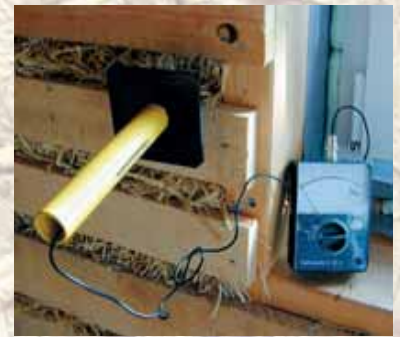
Measuring Moisture in Straw Bale Walls
