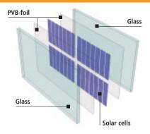
nated with the conventional EVA foil but rather with a PVB (polyvinyl-butyral) foil. Compared to conventional production technologies, this lamination method shows advantages with a view to tear resistance, breaking elongation, residual carrying capacity, and long-term behavior.
