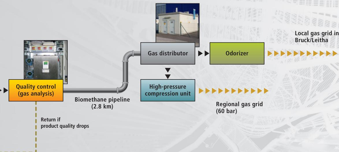
the new treatment unit has been fully integrated in the existing biogas facility in Bruck an der Leitha: the residual methane is not vented, but passed to the gas engines in the existing cogeneration units. This way the chemical energy in the off-gas is used to produce electricity and heat. The way in which the biomethane stream is then handled
