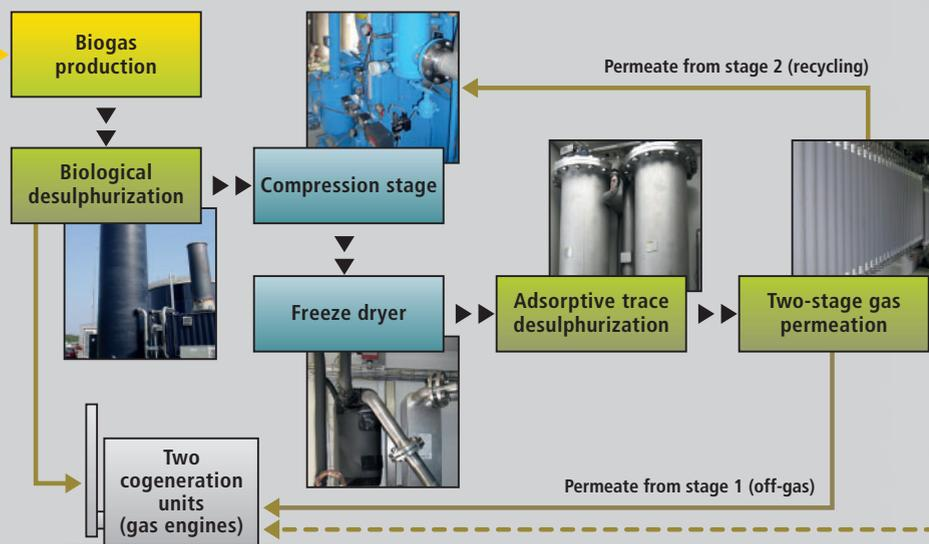
which contains significantly more methane than that from membrane stage 1, is returned and recompressed. The permeate from membrane stage 1 functions as a sink for the carbon dioxide involved, and leaves the treatment unit as off-gas. Like all other separation methods, gas permeation is unable to
