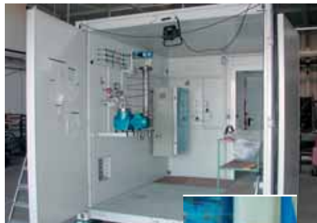
Container assembly, production of membrane modules from polyamide hollow fibers, Vienna University of Technology/ Department of Process Engineering
