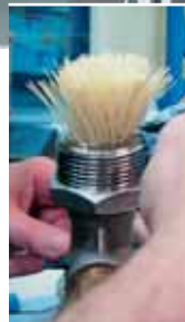
Container assembly, production of membrane modules from polyamide hollow fibers, Vienna University of Technology/ Department of Process Engineering
