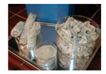
for the clean-up of contaminated soils is good; efficiency as hygienic material for animals has been shown to be very good (adsorptive capacity was 0.7 to 0.9 kg oil per kg of granular material and 1.0 to 1.3 kg water per kg of granular material). The product can, however, not be used as oil binder on water surfaces because it does not meet the requirements regarding buoyancy.
