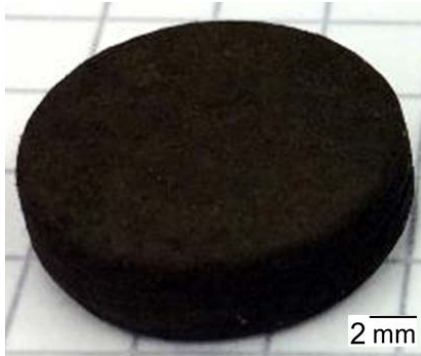
Mixed fibers and copper powder pressed at 100 MPa and carbonized
