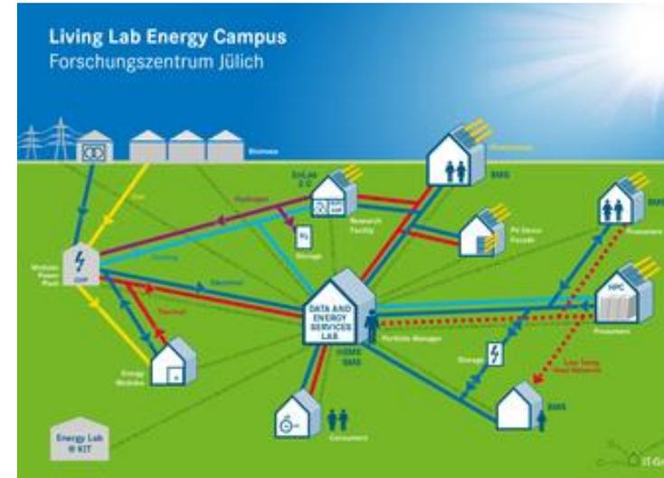
The basic idea of all projects in the LLEC is to link electrical, thermal and chemical energy flows in the plant network via a new intelligent IT system. For this purpose, part of the campus is transformed into real-life laboratory, where interactions between technology, energy sources and consumers, are investigated. Storage technologies used are Li-Ion batteries, compressed Hydrogen and LOHC storage for battery electric vehicle or hydrogen vehicle and heat distribution over grid.
