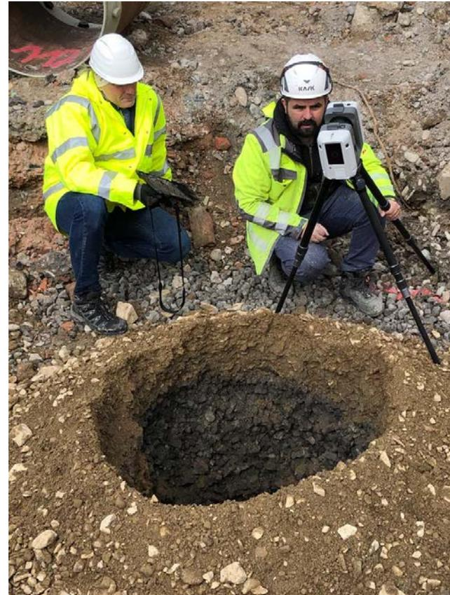
borehole laser scanning
