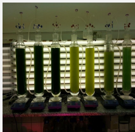
1.7 L Bubble columns with LED-tubes
