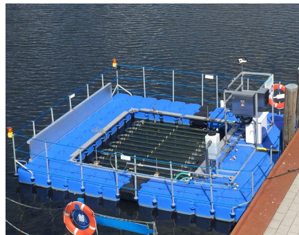
Figure 2: Floating pilot plant for microalgae cultivation on a channel in Harburg. Pipes can be immersed continuously into the surface water for temperature regulation.
