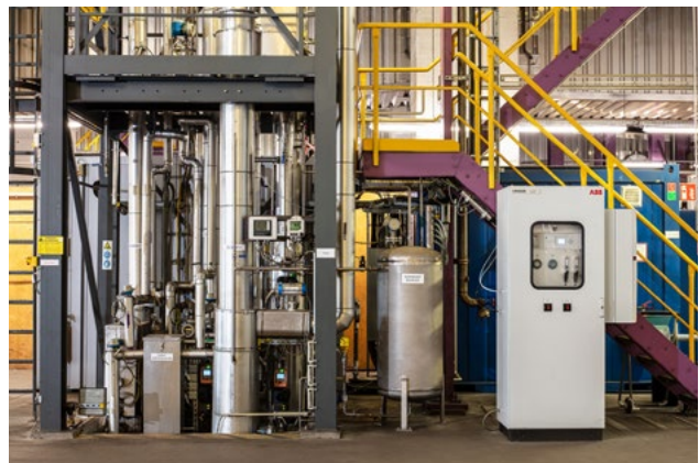
The plant uses an amine process to separate carbon dioxide from the flue gases resulting from iron production, photo: voestalpine Stahl GmbH
