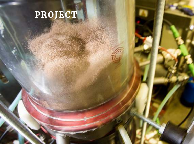
Detailed view of a fluidised bed, photo: TU Wien (Vienna University of Technology), Institute of Chemical Process Engineering and Energy Technology
