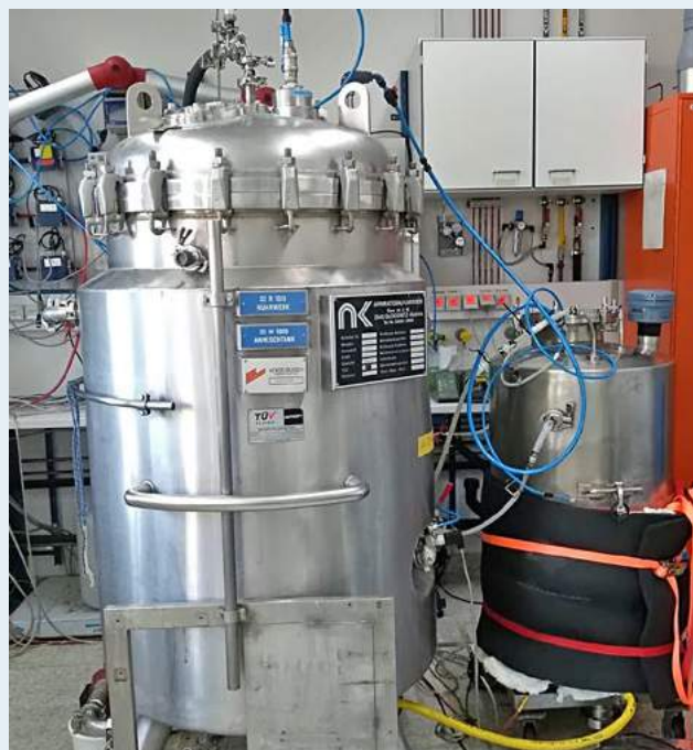
Bio-trickling reactor scale-up, photo: University of Natural Resources and Life Sciences, Institute of Environmental Biotechnology
