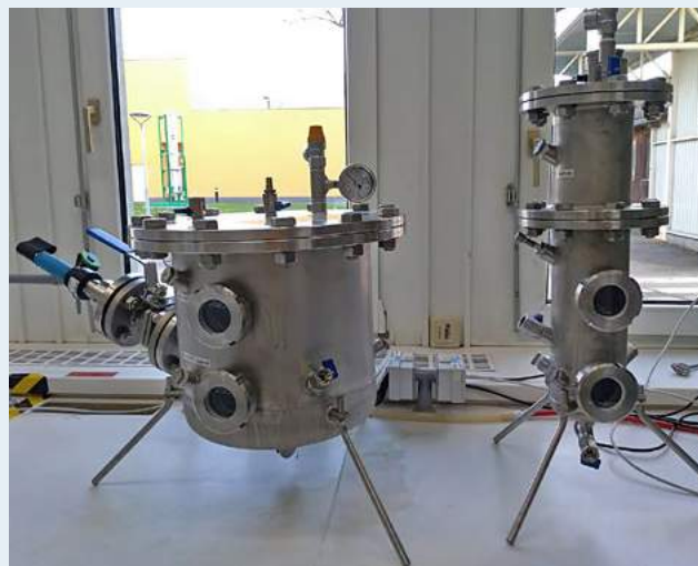
Bio-trickling filter and CSTR (Continuous stirred-tank reactor) at small scale, photo: University of Natural Resources and Life Sciences, Institute of Environmental Biotechnology
