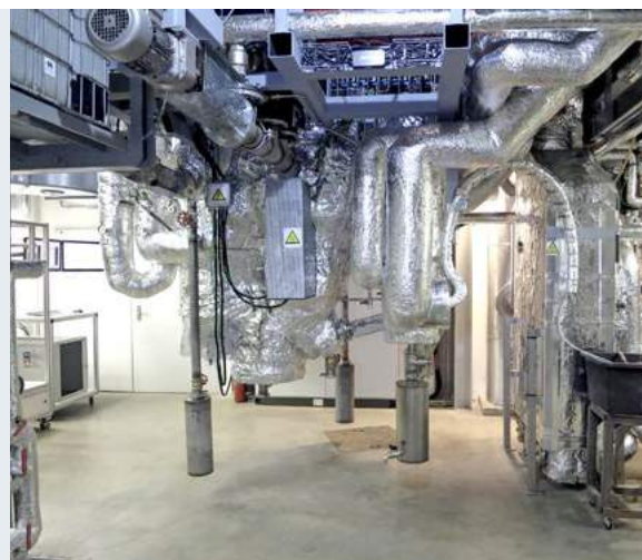
Fluidised bed test system for chemical looping combustion and biomass gasification, photo: TU Wien (Vienna University of Technology), Institute of Chemical Process Engineering and Energy Technology
