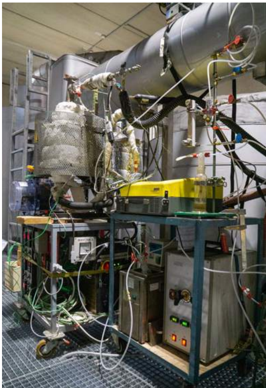
Test setup for adsorptive desulphurisation with online gas analysis (FTIR), photo: BEST / Lagler
