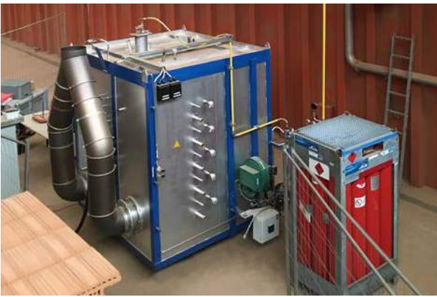
TOREtech hot test stand, photo: Wienerberger AG
