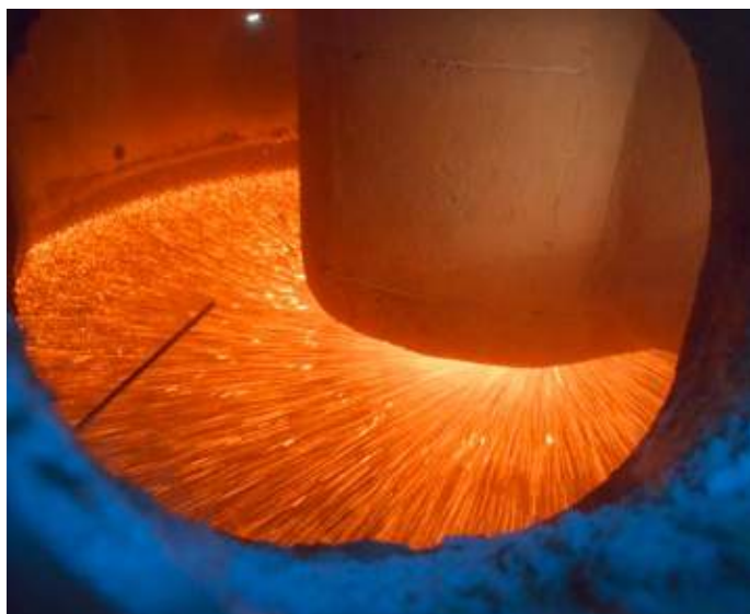
Above: Granulation in progress On left: Dry granulate photos: Primetals Technologies
