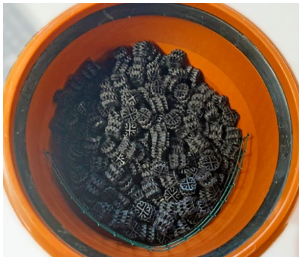
The investigations involved two trickle-bed reactors being built for biomethanation before they were put into operation at TU Wien. Each had a bulk volume of 17 litres and a total volume of 21.4 litres. Photos: TU Wien, Institute of Water Quality and Resource Management
