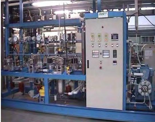
Abb. 45 SFE-Anlage (Supercritical Fluid Extraction) © NATEX
