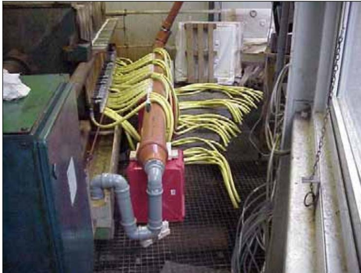
**Fig 5:** Devices to measure the time characteristic of compressed air amount and dehydration process in single filter cells
