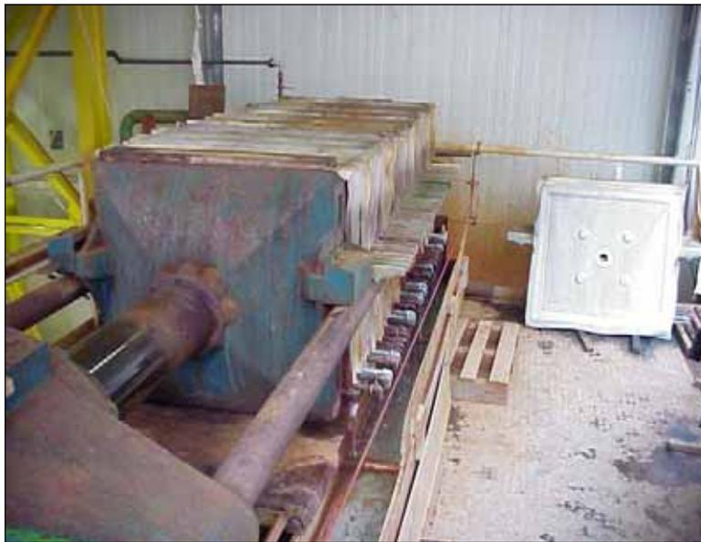
Fig. 1: Cell filter press
