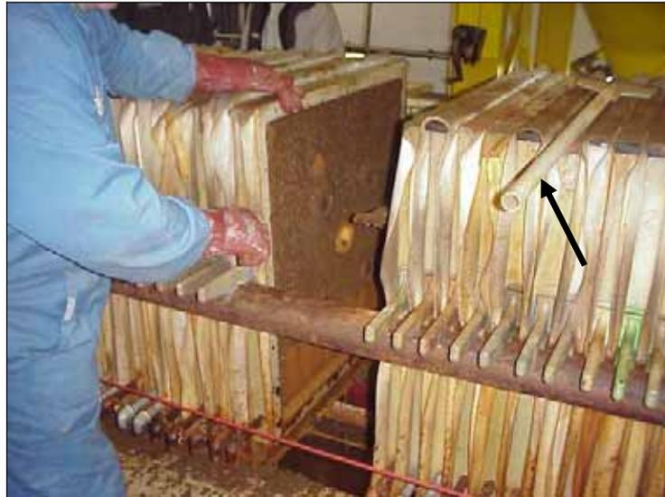
Fig. 3: Manual removal of the filter residues from the filter mat by shaking of the filter mats, or if necessary with a scraper (see arrow)
