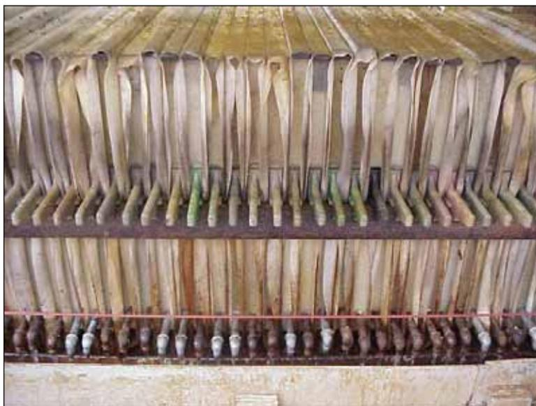
Fig. 2: Cell filter press; side view of the cell plates
