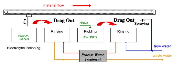
Figure 3: Possible measures to reduce water and chemical consumption.
