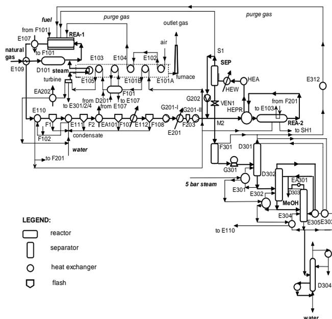
Figure 2: Process flow diagram of a low-pressure Lurgi methanol plant.
