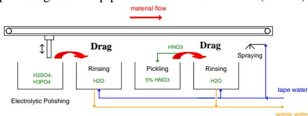
Figure 1: Electro Polishing Process
