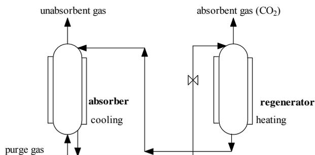
Figure 1: Basic flow sheet for absorption system.
