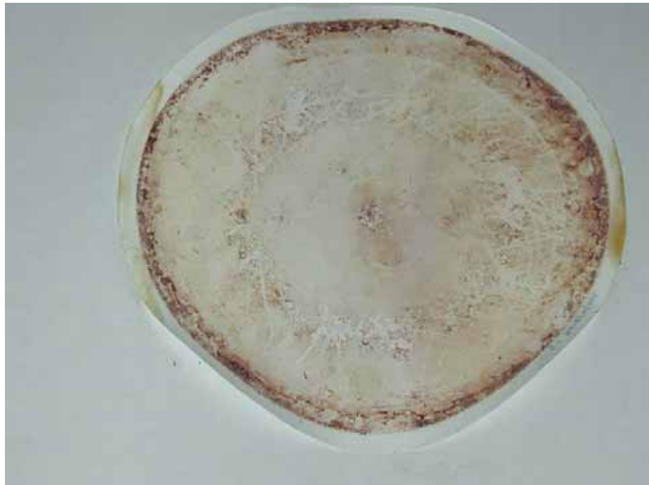
Abb. 48: Nanofiltrationsmembran NADIR PES 10 (nominaler cut-off 1 kD)
