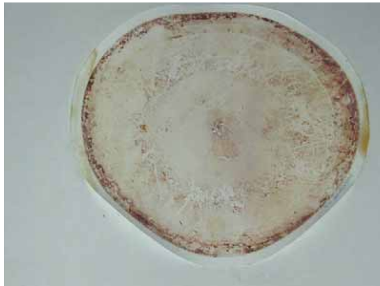
Abb. 13: Nanofiltrationsmembran NADIR PES 10 (nominaler cut-off 1 kD)
