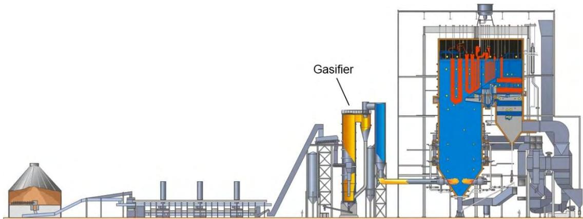
**Figure 5-5** Vaskiluodon Voima biomass gasification facility. Metso Power Oy gasifier with fuel pre-treatment equipment and dryer connected to a coal-fired power plant in Vaasa, Finland was commissioned in the end of the year 2012 [72].
