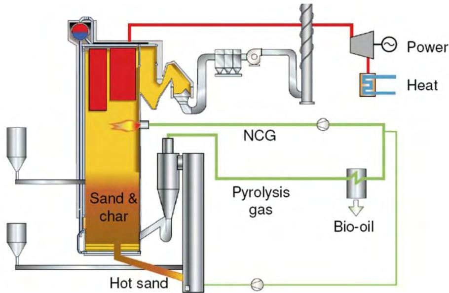
**Figure 5-3.** Integrated pyrolyser by VTT, Metso, UPM and Fortum [65].
