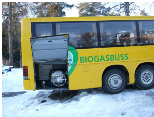
Figure 1 A biogas bus for public transportations with the biogas tank in the cargo area (Photo: Kalle Svensson, Sweden Energy Agency)
