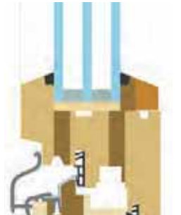
↑ Illustration 213 : Frame in wood and cork
