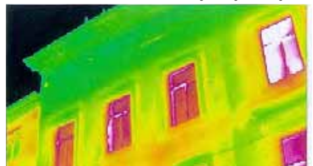
↓ Illustration 143 : Thermal bridges during the heating season
