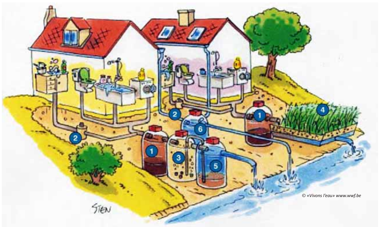
↑ Illustration 387 : The difference between mechanical system and plants system (intensive or extensive system)
