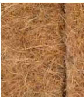
↑ Illustrations 160, 161, 162 and 163: Natural fibers insulation : coconut fibers, wood fibers, cork and sheep wool
