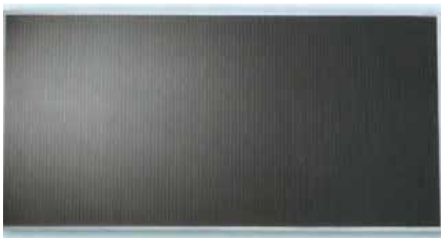
↑ Illustration 311 : Cell with amorphous silicon
