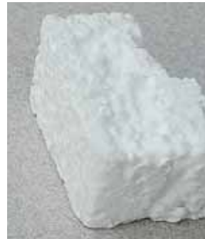
↑ Illustrations 158 and 159: Insulation coming from petrochemical industry : EPS and PUR
