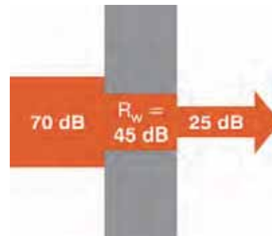
↑ Illustration 104: Illustration of the Mass principle
