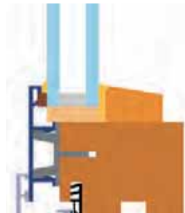
↑ Illustration 212: Frame in wood and aluminium
