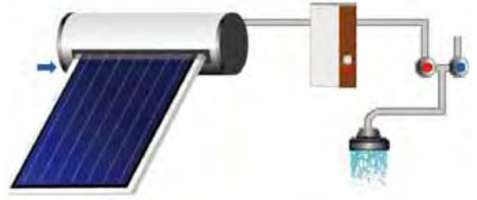
Figure 45: Hydraulic scheme of the domestic hot water thermosiphon reference system for single family houses
