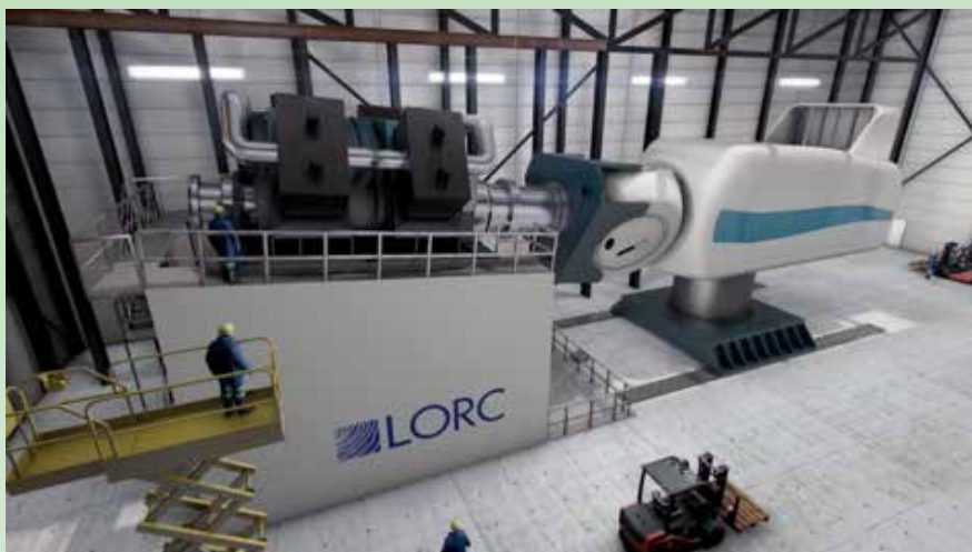
Figure 5. The HALT Tester of LORC Nacelle Testing - 6 degrees of freedom loads
