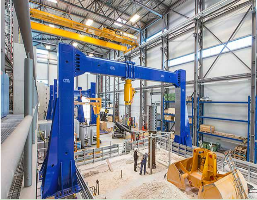
Figure 3. ForWind's test center support structures (Source: Faculty of Civil Engineering and Geodetic Science, Leibniz Universität Hannover)
