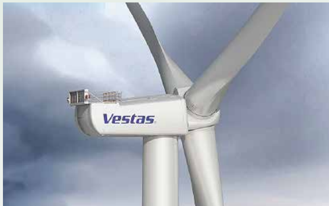
Figure 4. Vestas 8-MW wind turbine (Courtesy of Vestas Wind Systems A/S)
