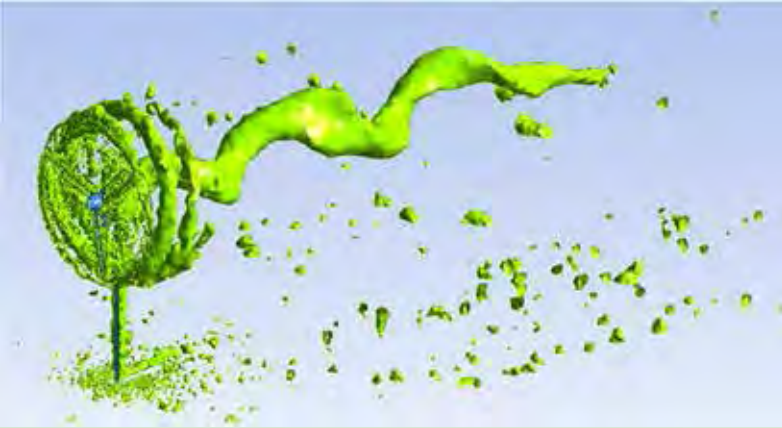
Figure 3. The vortex in the wake of a wind turbine
