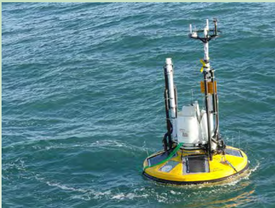
Figure 4. The Met Ocean Buoy with lidar being developed under the FLOW program
