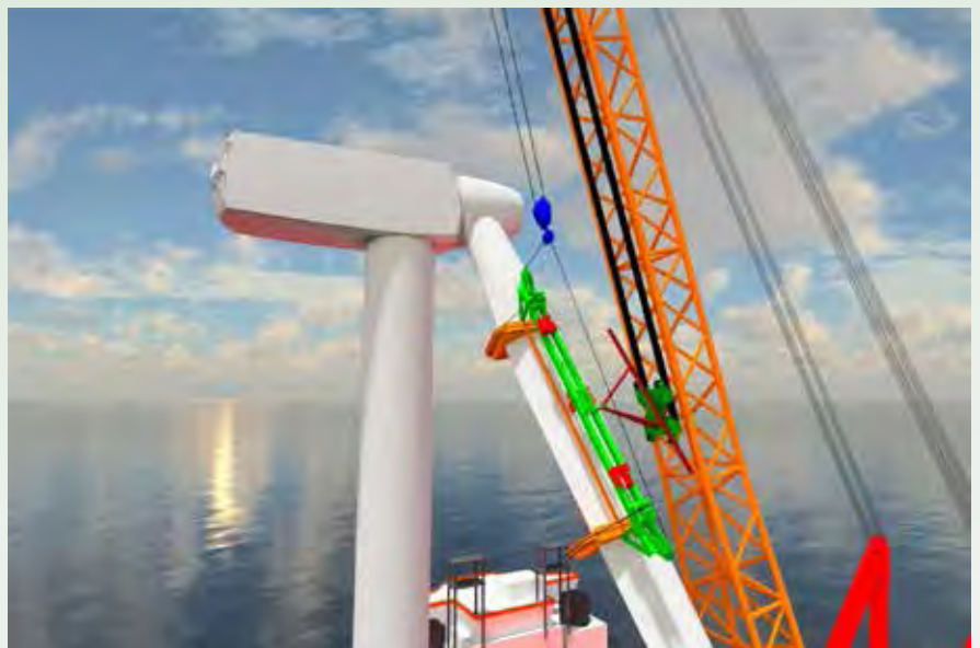
Figure 3. Art impression of the boom based blade manipulator, being designed and developed under the FLOW program
