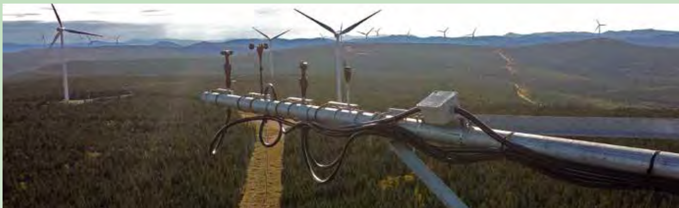
Figure 1. Anemometer and wind vane boom for wind farm studies (credit: NRCan)
