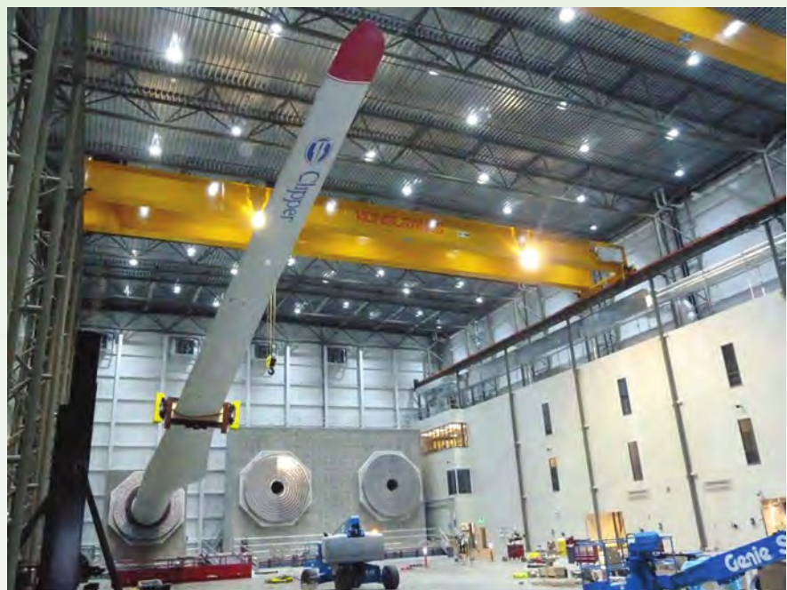
Figure 3. A 46.7-m blade undergoing commissioning tests at the new Wind Technology Testing Center in Boston, Massachusetts (Source: NREL/PIX 19939)
