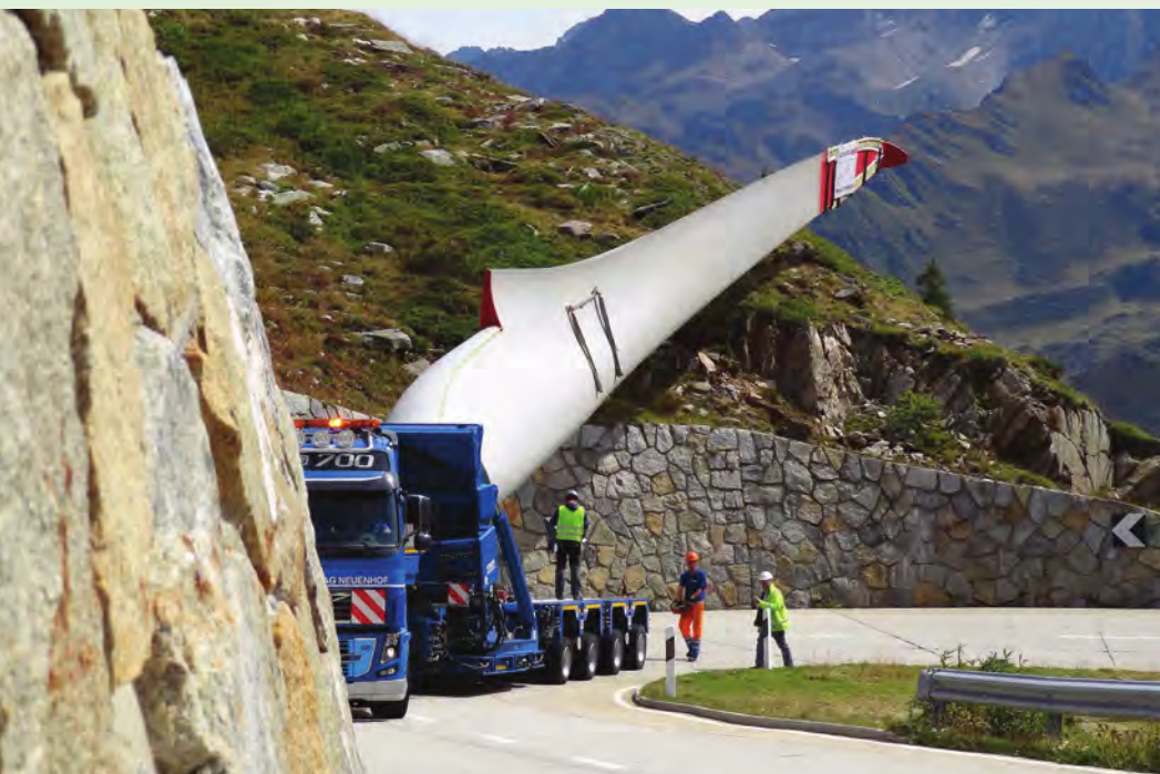
Figure 4. Transport solutions for difficult access in mountainous areas, e.g., tilting blade adapter
