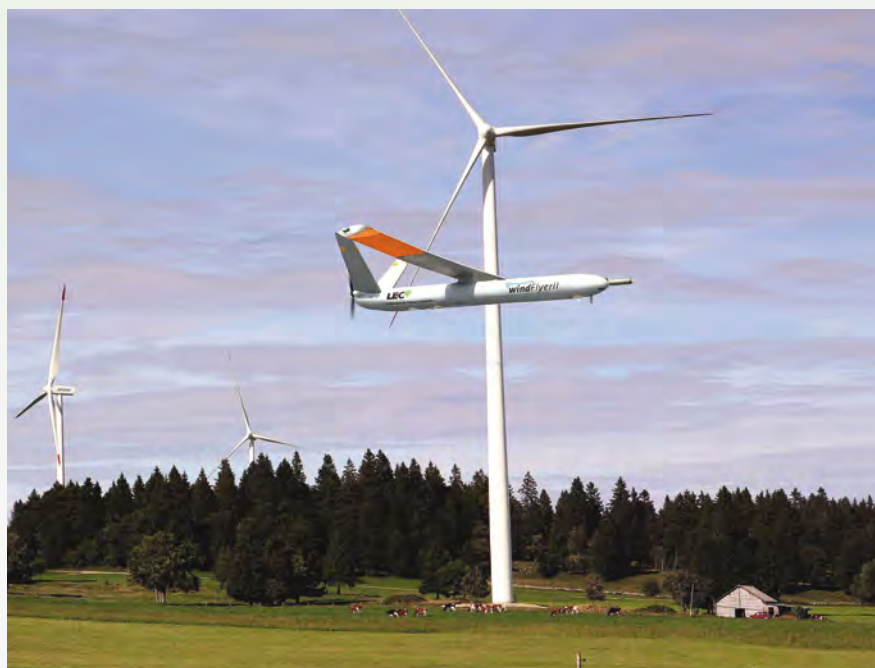
Figure 3. The novel approach of using an instrumented Unmanned Aerial Vehicle (UAV) to measure the wind speed and turbulence in wind parks has been developed at ETH Zürich
