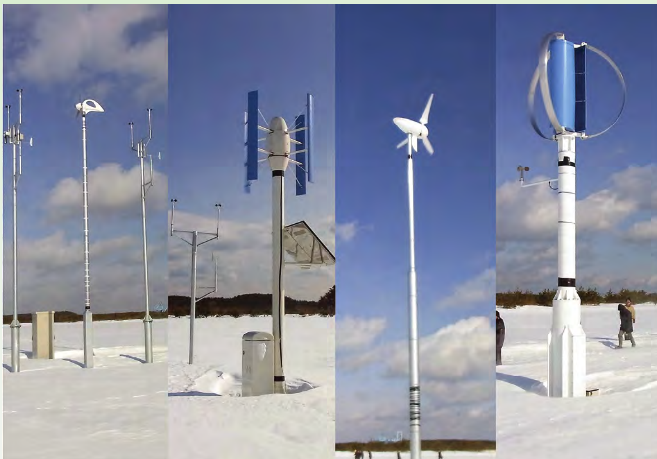
Figure 3. Field test site for small wind turbines in Rokkasho, Aomori (From left to right, Nasu Denki-Tekko "Aura 1000", Sinfonia Technology "V-II WK18-20", Nikko "NWG-1K", Mayekawa "MDS-01A") (Photo credit: HIKARUWIND.LAB)
