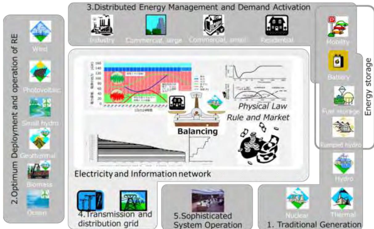
Figure 2.5-1: The enhanced power system operation by optimized utilization of the whole resources of flexibility against the smoothed variability Source: Ogimoto, Laboratory.
