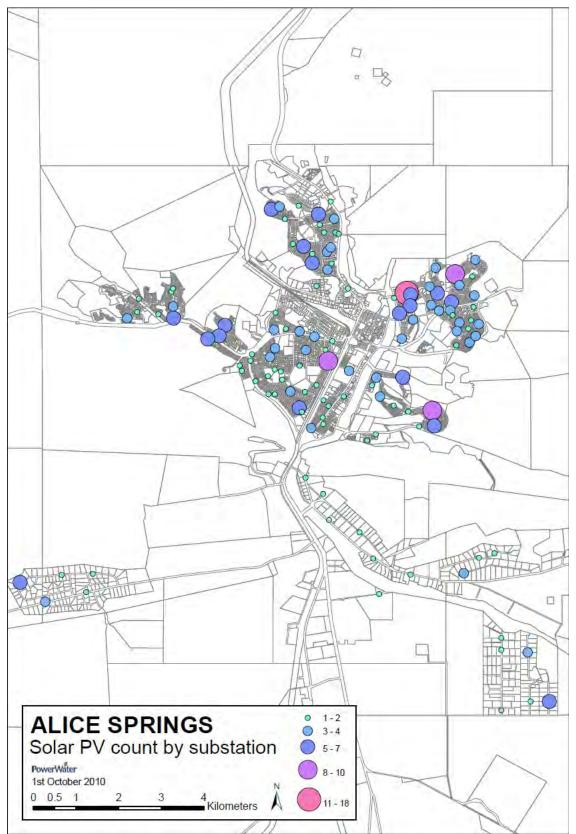
Figure 8: Diagram of PV system distribution on the Alice Springs Network (status: 10/2010)
