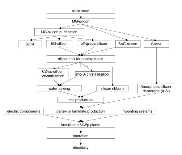
Figure 10 Supply chain of silicon based photovoltaic electricity production. MG-silicon: metallurgical grade silicon; EG-silicon: electronic grade silicon; SoG-silicon: solar-grade silicon; a-Si: amorphous silicon; CZ: Czochralsky; kWp: kilowatt peak (according to Jungbluth et al. (2012) [38]).
