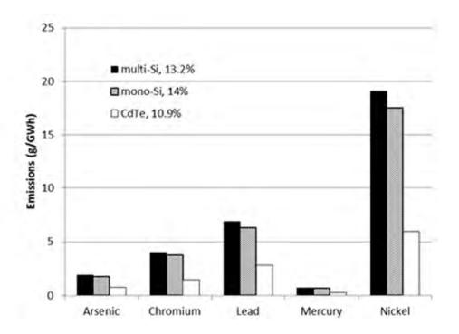
Figure 9: Emissions of heavy metals due to electricity use, based on European ENTSO-E average (ecoinvent database). Emissions are normalized for Southern European average insolation of 1700 kWh/m2/yr, performance ratio of 0.8, and lifetime of 30 yrs. Each PV system is assumed to include the ground-mounted BOS (Mason et al. [13]).
