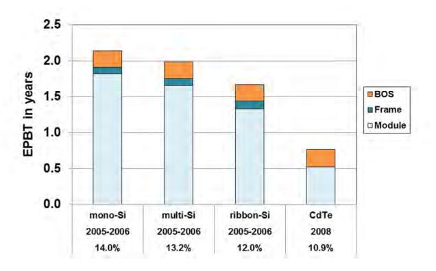
Figure 2: Energy payback time (EPBT) of rooftop mounted PV systems estimated from the currently available LCI data for European production and installation. The estimates are based on Southern European irradiation of 1700 kWh/m2/yr and performance ratio of 0.75. See Tables 5.1.1-5.2.3, 5.4.1, and 5.5.1.1-5.5.1.4 for the corresponding LCI data.
