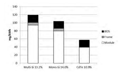
Figure 7: Life-cycle SO<sub>2</sub> emissions from silicon and CdTe PV modules, wherein BOS is the Balance of System (i.e., module supports, cabling and power conditioning). The estimates are based on rooftop-mount installation, Southern European insolation, 1700 kWh/m2/yr, a performance ratio of 0.75, and a lifetime of 30 years. It is assumed that the electricity supply for all the PV system is from the ENTSO-E grid.
