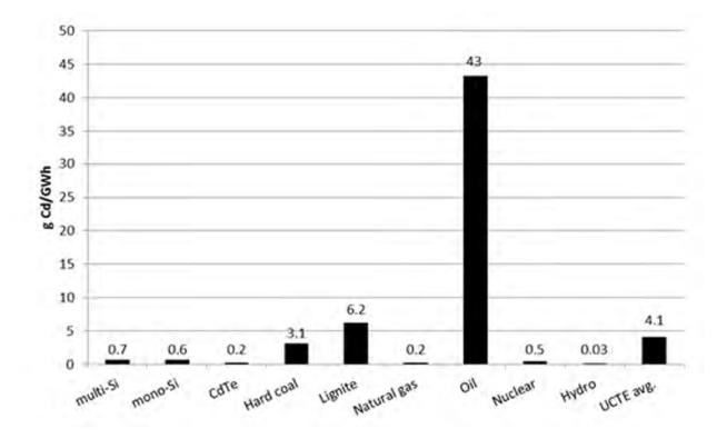
Figure 8: Life cycle atmospheric Cd emissions for PV systems from electricity and fuel consumption, normalized for a Southern Europe average insolation of 1700 kWh/m2/yr, performance ratio of 0.8, and lifetime of 30 yrs. A ground-mounted BOS is assumed for all PV systems [12].
