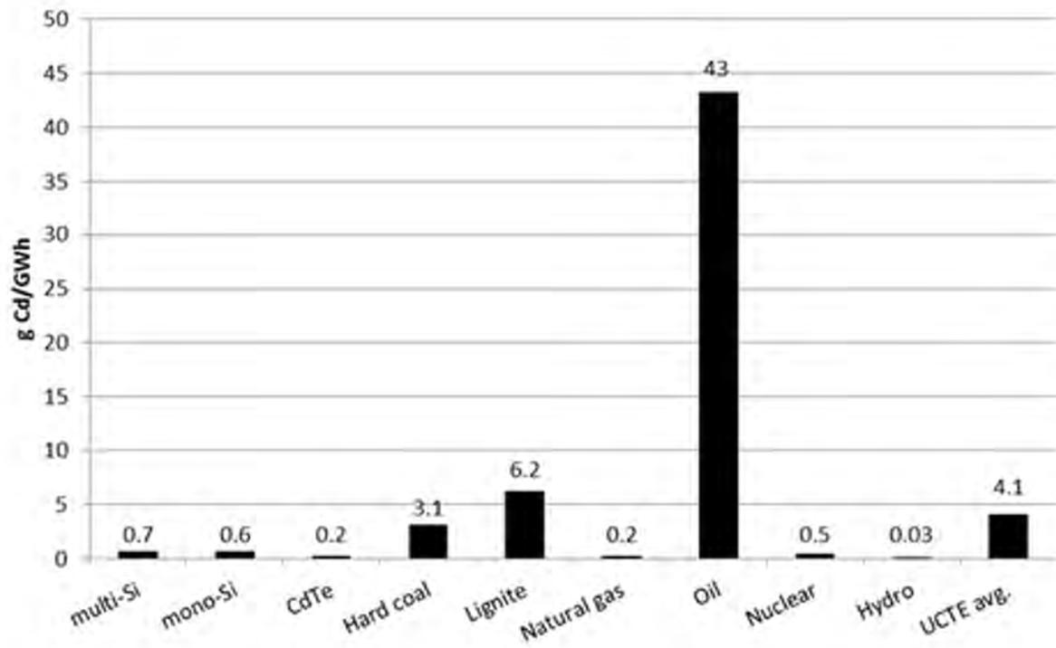
Figure 8: Life cycle atmospheric Cd emissions for PV systems from electricity and fuel consumption, normalized for a Southern Europe average insolation of 1700 kWh/m<sup>2</sup>/yr, performance ratio of 0.8, and lifetime of 30 yrs. A ground-mounted BOS is assumed for all PV systems [12].
