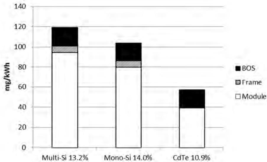
Figure 7: Life-cycle  $\text{SO}_2$  emissions from silicon and CdTe PV modules, wherein BOS is the Balance of System (i.e., module supports, cabling and power conditioning). The estimates are based on rooftop-mount installation, Southern European insolation,  $1700 \text{ kWh/m}^2/\text{yr}$ , a performance ratio of 0.75, and a lifetime of 30 years. It is assumed that the electricity supply for all the PV system is from the ENTSO-E grid.
