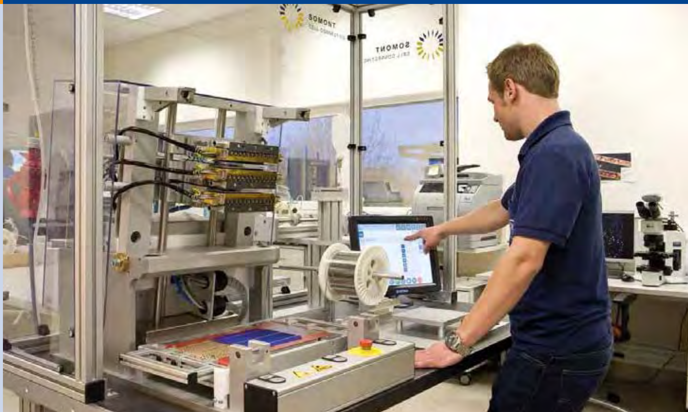
Fig. 2 - Simulation of solar cell stringing for development of new interconnect materials, Ulbrich Solar Technologies.
