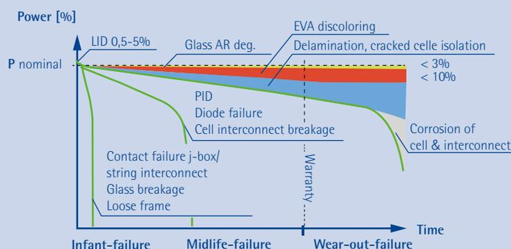
Fig. 3 - Three typical failure scenarios for wafer based crystalline photovoltaic modules are shown. Definition of the used abbreviations: LID - Light Induced Degradation, PID - Potential Induced Degradation, EVA - Ethylene Vinyl Acetate, j-box - junction box (Diagram: Marc Köntges, ISFH).
