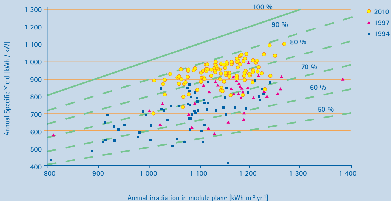
Fig. 2 – Monitored specific energy yields as a function of total plane-of-array irradiances of PV systems installed in Germany during the years 1994, 1997, and 2010. Clearly, specific energy yields have been improved during the past 17 years (from: Reich et al. Prog. Photovolt. 20 (2012) 717-726).
