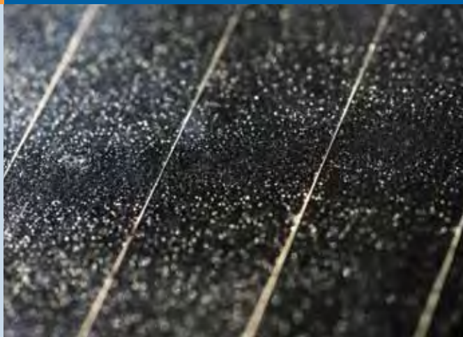
Fig. 2 - Flexible CZTS photovoltaic film (for integration into building elements) (Photo: crystalsol).
