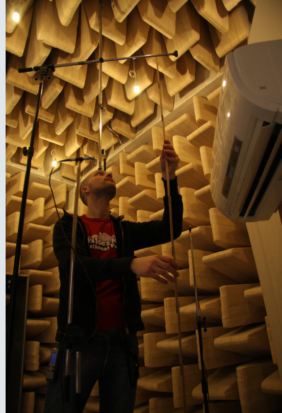
Figure 1. Noise measurement of an air-to-air heat pump in the hemi-anechoic room at RISE in Sweden. [Source: RISE Research Institutes of Sweden]
