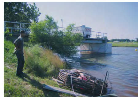
An instrumented surface water heat exchanger about to be moved into a pond. (source: Oklahoma State University)
